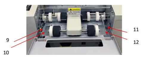
9 & 11. Paper Thickness Adjustment Needle
