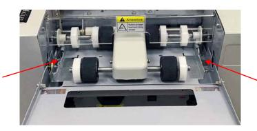
Paper Thickness Adjustment Needle
